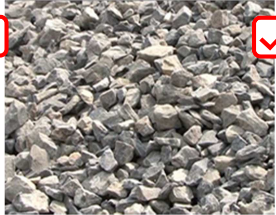
Well graded angular aggregate
