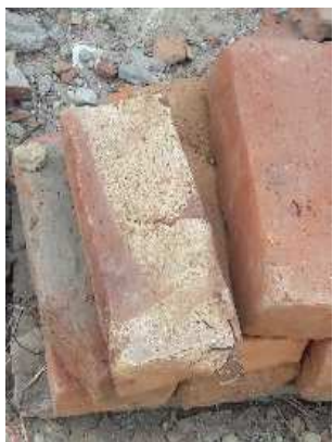
Over burned / irregular bricks
