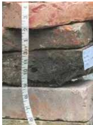
Over burned / irregular bricks
