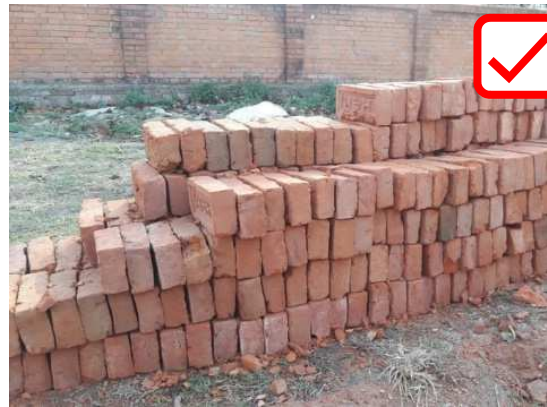
Bricks uniformly burned
